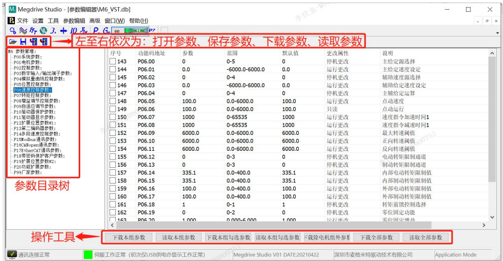
Attached Fig.B-11 Parameter editing function introduction
