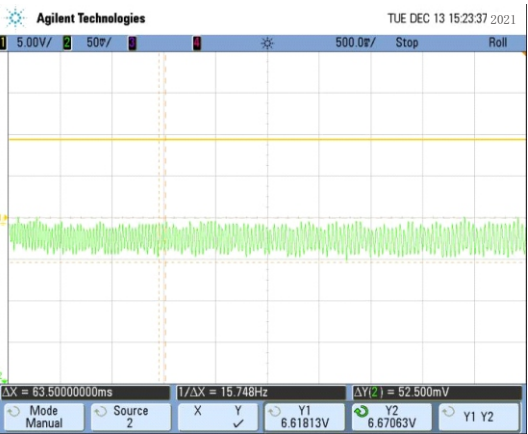
Pressure sensor range 250bar, 0 ~ 10V output. Hold pressure 175bar, pressure fluctuations is ± 0.65kg / cm2.
