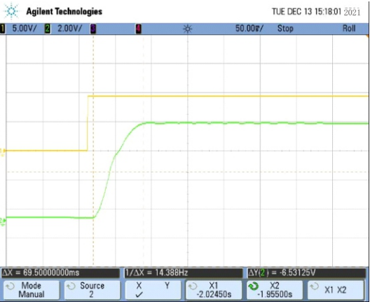
Building pressure time of 175bar is 64.5ms.
