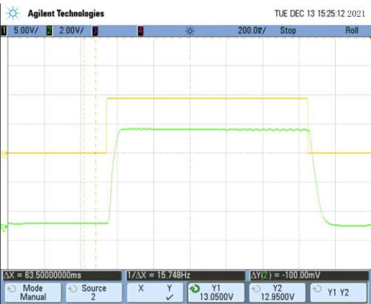
Fast response to cyclical building pressure, hold pressure, unloading pressure instructions.
