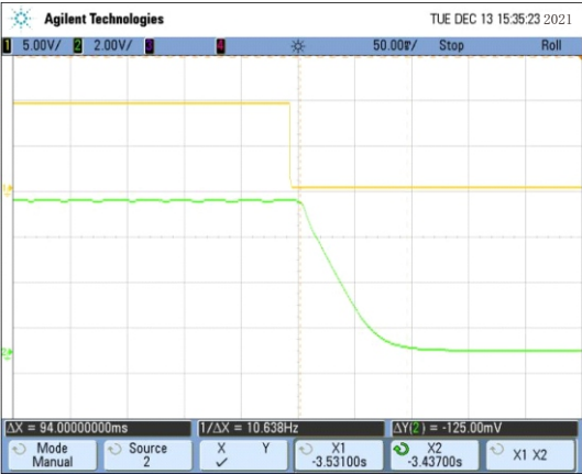
Unloading pressure time of 175 bar is less than 100ms.
