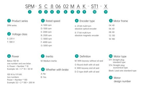
Fig.1-1 M5 servo motor model
