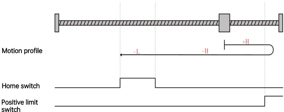
The present motor position is in the effective zone of the home switch. When homing starts, the home switch is at a high level, and homing is processed in the backward direction at a low speed. Homing stops when the motor reaches the falling edge of the home switch.
