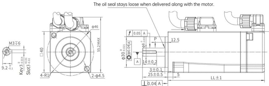
Fig. 2-3 Frame No. 40 servo motor dimensions
