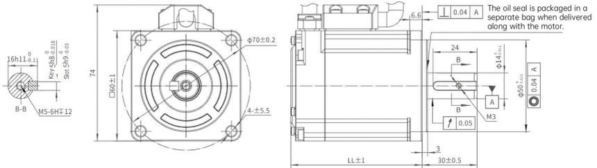
Fig. 2-4 Frame No. 60 servo motor dimensions (without brake)
