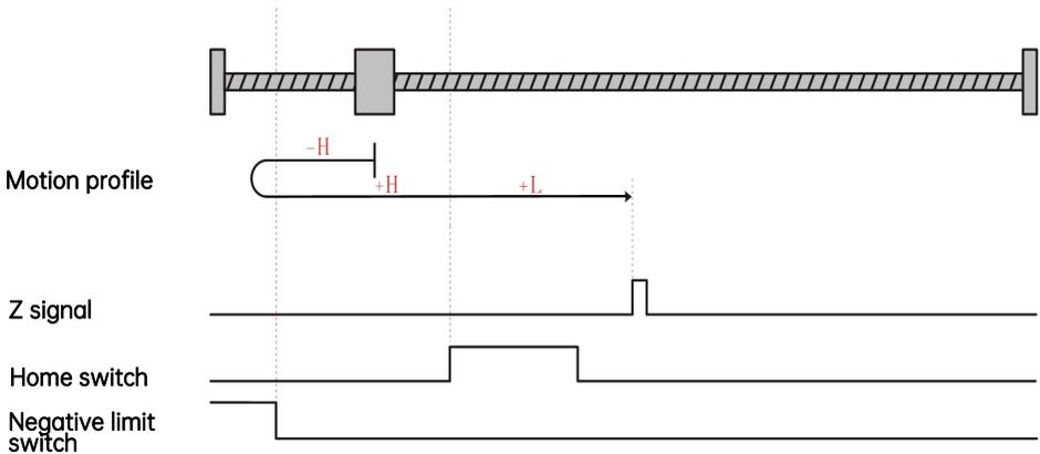
The present motor position is in the effective zone of the home switch. When homing starts, the home switch is at a high level, and homing is processed in the forward direction at a low speed. Homing stops when the motor reaches the rising edge of the Z signal.
