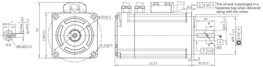
Fig. 2-5 Frame No. 60 servo motor dimensions (with brake)
