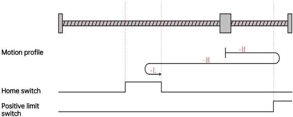
The present motor position is in the effective zone of the home switch. When homing starts, the home switch is at a high level, and homing is processed in the forward direction at a low speed. Homing stops when the motor reaches the falling edge of the home switch.
