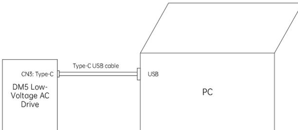
2. Start the software **M. Driver.Soft.exe**, select "DM5" in "Servo Serial", select the correct serial port number, and click "Connect" in the "Communication Config" interface.
