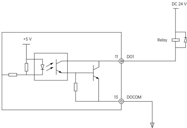
Fig. 4-6 Wiring between the DO terminal and the relay
