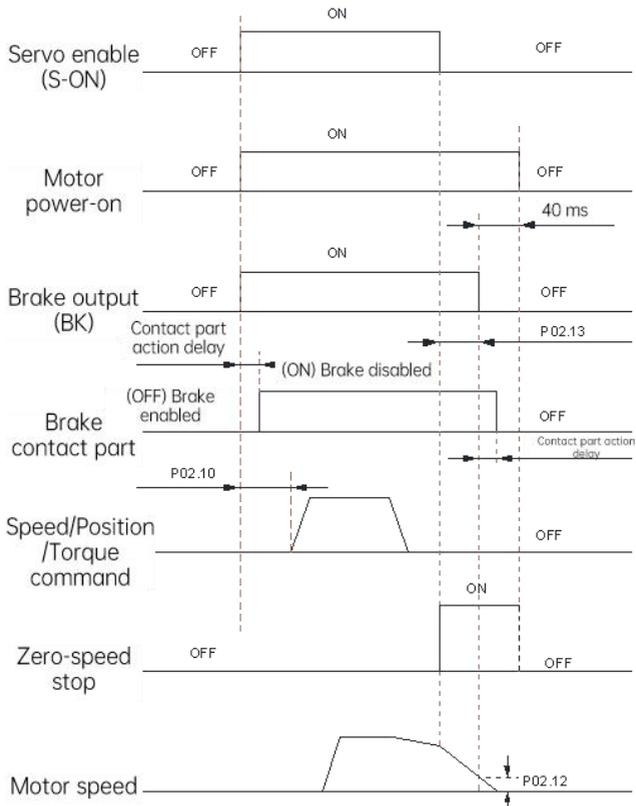
Fig. 5-5 Brake time sequence for rotating motor
