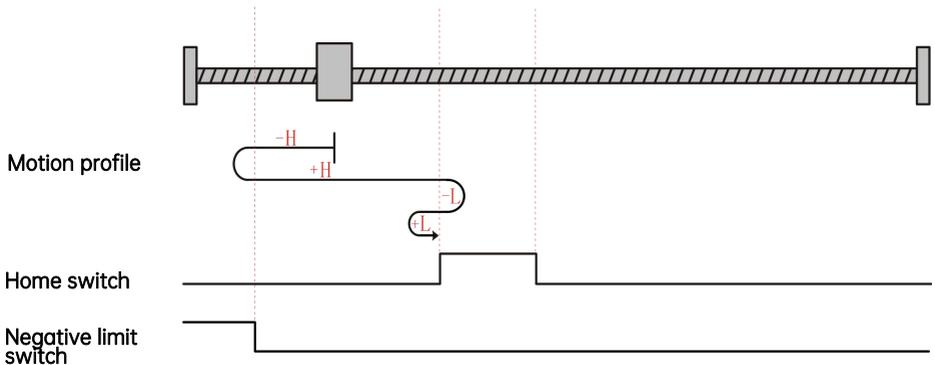
The present motor position is in the effective zone of the home switch. When homing starts, the home switch is at a high level, and homing is processed in the backward direction at a low speed till it reaches the falling edge of the home switch. Then, homing is processed in the forward direction at a low speed,
