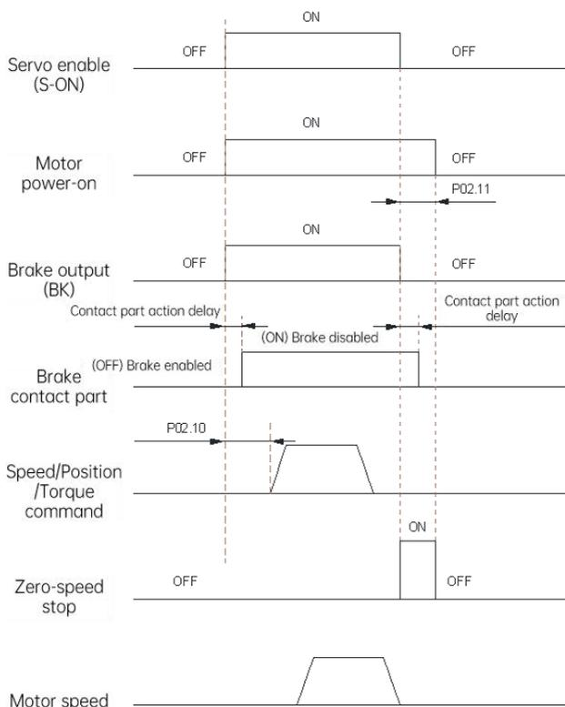
Fig. 5-4 Brake time sequence for static motor
