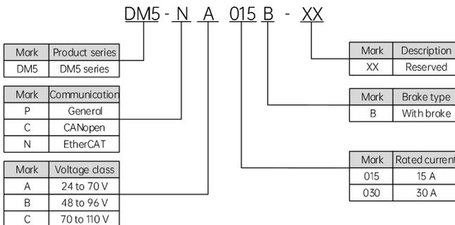
Fig. 1-3 DM5 Servo drive model
