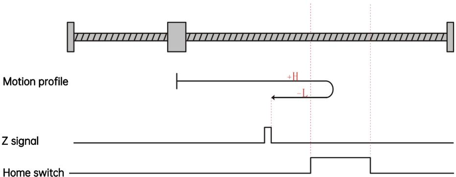
The present motor position is in the effective zone of the home switch. When homing starts, the home switch is at a high level, and homing is processed in the backward direction at a low speed till it reaches the falling edge of the home switch. Then, homing continues in the backward direction at a low speed, and stops when the motor reaches the rising edge of the Z signal.
