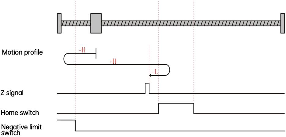
The present motor position is in the effective zone of the home switch. When homing starts, the home switch is at a high level, and homing is processed in the backward direction at a low speed. Homing stops when the motor reaches the rising edge of the Z signal.
