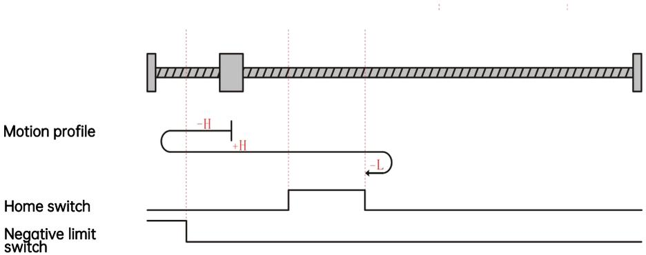
The present motor position is in the effective zone of the home switch. When homing starts, the home switch is at a high level, and homing is processed in the forward direction at a high speed till it reaches the falling edge of the home switch. Then, homing is processed in the backward direction at a low speed, and stops when the motor reaches the rising edge of the home switch.
