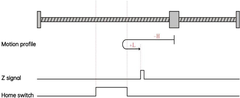
The present motor position is in the effective zone of the home switch. When homing starts, the home switch is at a high level, and homing is processed in the forward direction at a low speed till it reaches the falling edge of the home switch. Afterwards, homing continues in the forward direction at a low speed, and stops when the motor reaches the rising edge of the Z signal.
