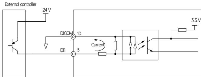
Fig. 4-5 PNP mode wiring of the DI terminal
