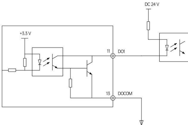
Fig. 4-7 DO terminal sink (NPN) output wiring mode
