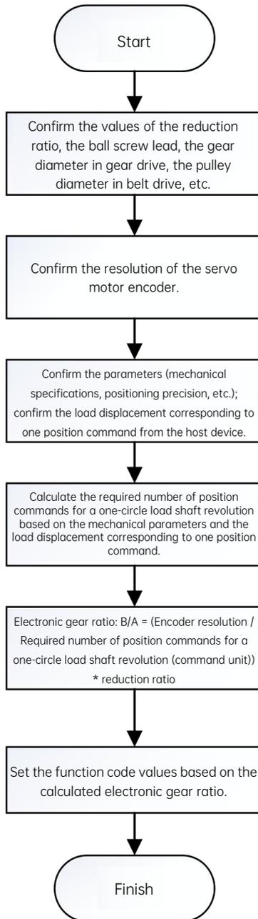
Fig. 5-1 Procedure for the electronic gear ratio setting
