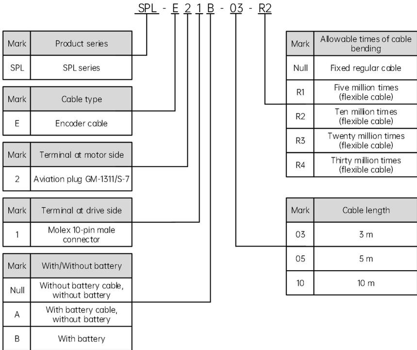
Fig. 1-8 Encoder cable selection
