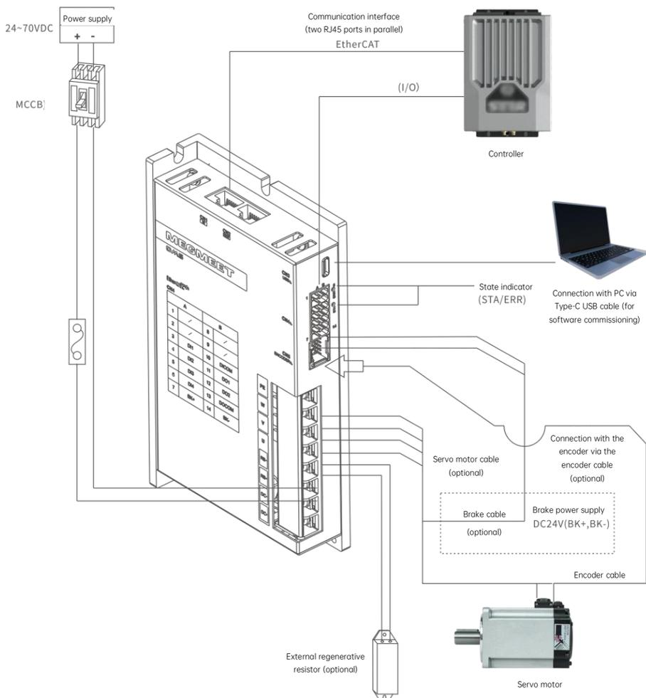
Fig. 3-3 SIZE B model wiring diagram
