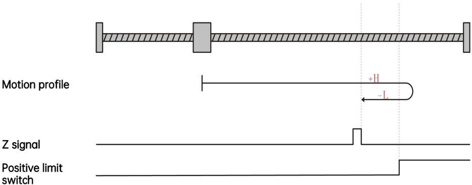
The present motor position is in the effective zone of the positive limit switch. When homing starts, the positive limit switch is at a high level, and homing is processed in the backward direction at a low speed till it reaches the falling edge of the positive limit switch. Then, homing continues in the backward direction at a low speed, and stops when the motor reaches the rising edge of the Z signal.
