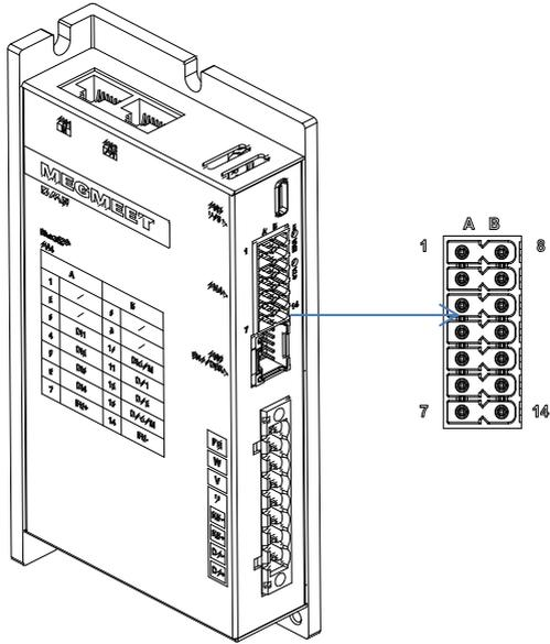
Fig. 4-2 Control signal terminal definition
