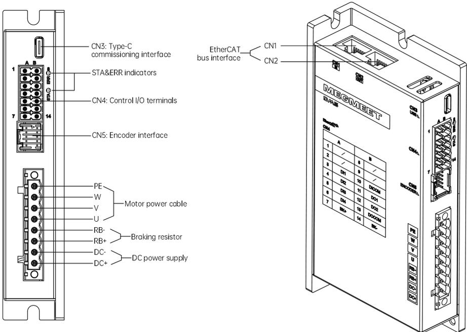
Fig. 1-5 DM5-N servo drive drawing (SIZE A)
