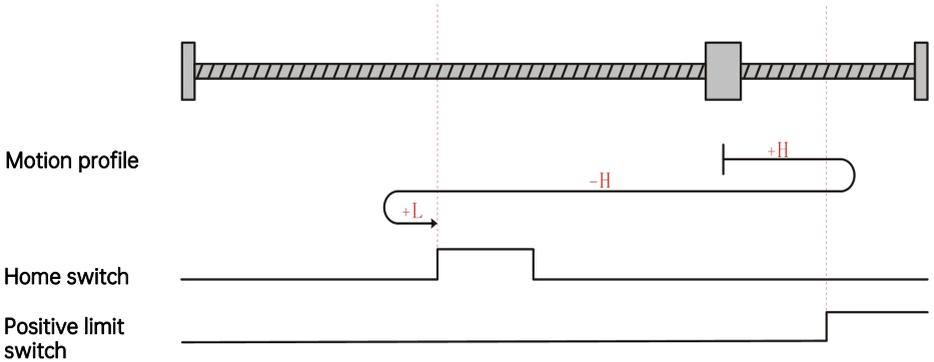
The present motor position is in the effective zone of the home switch. When homing starts, the home switch is at a high level, and homing is processed in the backward direction at a high speed till it reaches the falling edge of the home switch. Then, homing is processed in the forward direction at a low speed, and stops when the motor reaches the rising edge of the home switch.
