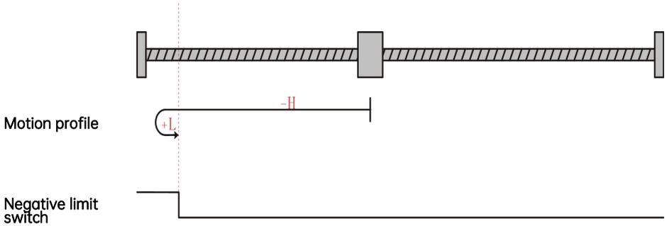
The present motor position is in the effective zone of the negative limit switch. When homing starts, the negative limit switch is at a high level, and homing is processed in the forward direction at a low speed. Homing stops when the motor reaches the falling edge of the negative limit switch.
