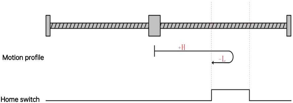
The present motor position is in the effective zone of the home switch. When homing starts, the home switch is at a high level, and homing is processed in the backward direction at a low speed. Homing stops when the motor reaches the falling edge of the home switch.
