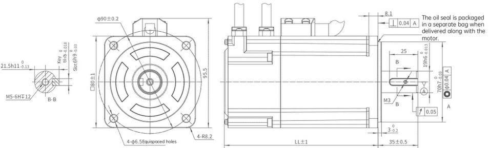
Fig. 2-7 Frame No. 80 servo motor dimensions (with brake)
