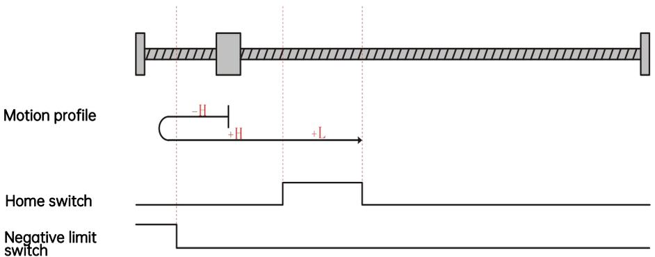
The present motor position is in the effective zone of the home switch. When homing starts, the home switch is at a high level, and homing is processed in the forward direction at a low speed. Homing stops when the motor reaches the falling edge of the home switch.
