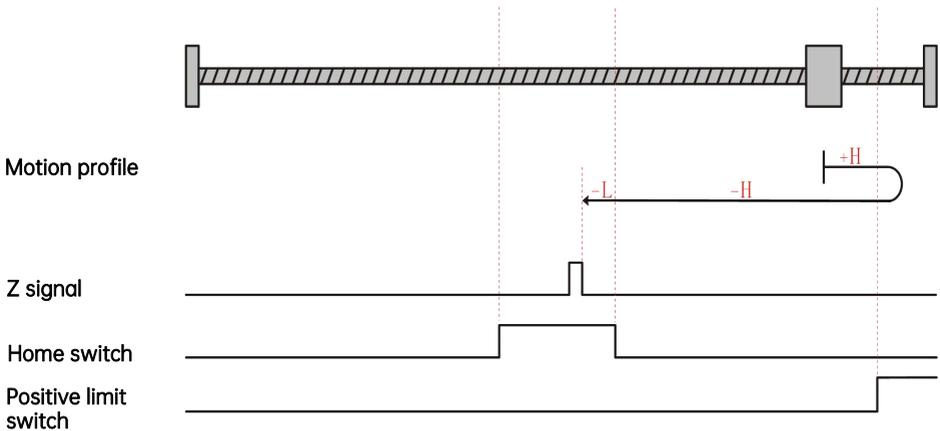
The present motor position is in the effective zone of the home switch. When homing starts, the home switch is at a high level, and homing is processed in the forward direction at a high speed till it reaches the falling edge of the home switch. Then, homing is processed in the backward direction at a high
