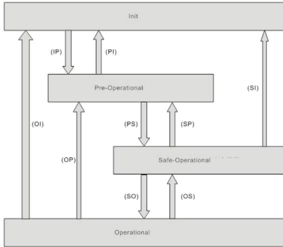
The EtherCAT state machine must support the following four states and coordinate the states of the master and slave application programs during initialization and operation.
