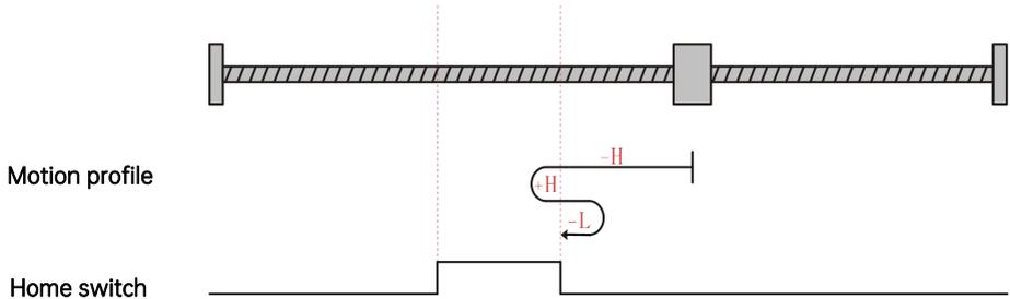
The present motor position is in the effective zone of the home switch. When homing starts, the home switch is at a high level, and homing is processed in the forward direction at a high speed till it reaches the falling edge of the home switch. Then, homing is processed in the backward direction at a low speed, and stops when the motor reaches the rising edge of the home switch.
