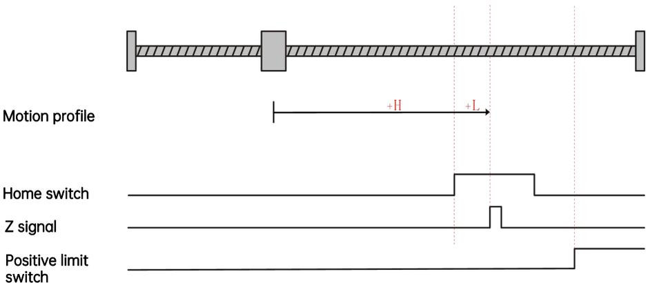
The present motor position is in the effective zone of the home switch. When homing starts, the home switch is at a high level, and homing is processed in the backward direction at a high speed till it reaches
