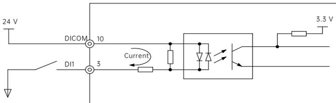
Fig. 4-3 Dry contact mode wiring of the DI terminal
