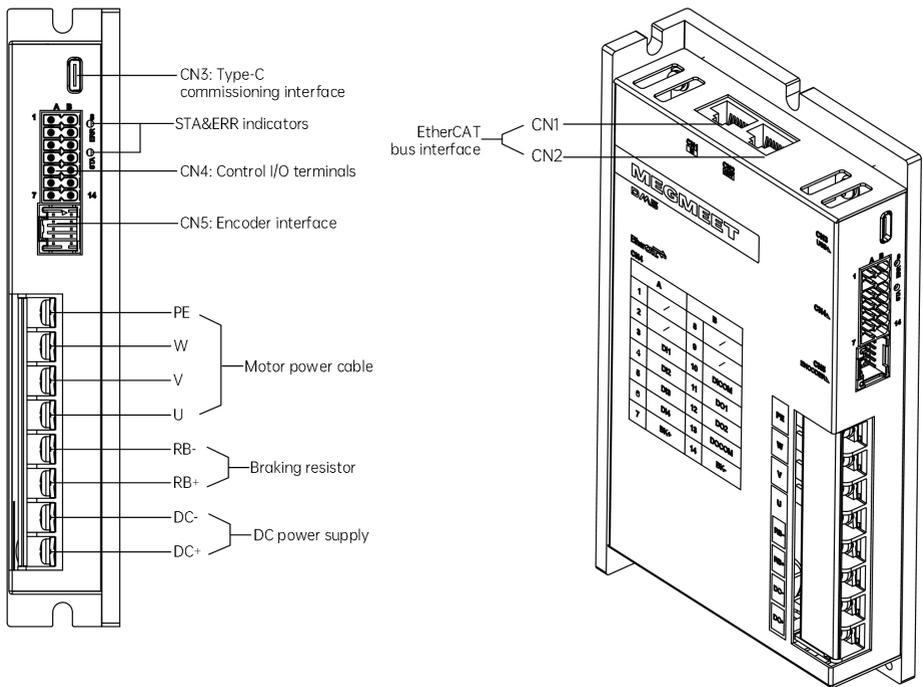
Fig. 1-6 DM5-N servo drive drawing (SIZE B)
