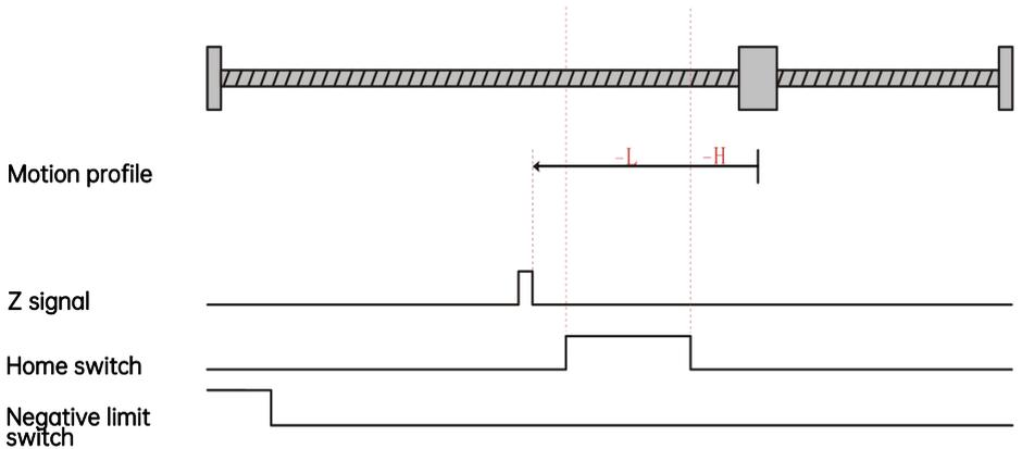
The present motor position is between the negative limit switch and the home switch. When homing starts, the home switch is at a low level, and homing is processed in the backward direction at a high speed till it reaches the rising edge of the negative limit switch. Then, homing is processed in the forward direction
