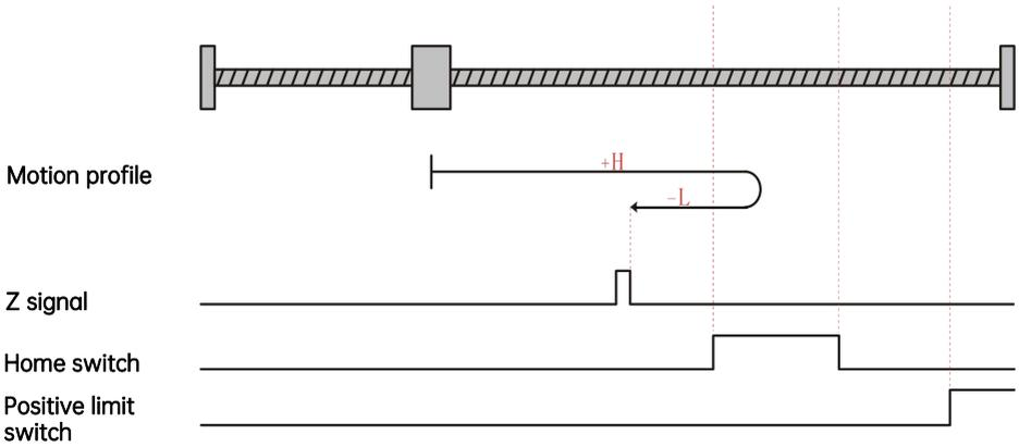
The present motor position is in the effective zone of the home switch. When homing starts, the home switch is at a high level, and homing is processed in the backward direction at a low speed till it reaches the falling edge of the home switch. Then, homing continues in the backward direction at a low speed, and stops when the motor reaches the rising edge of the Z signal.
