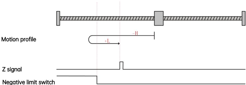
The present motor position is in the effective zone of the negative limit switch. When homing starts, the negative limit switch is at a high level, and homing is processed in the forward direction at a low speed till it reaches the falling edge of the negative limit switch. Then, homing continues in the forward direction at a low speed, and stops when the motor reaches the rising edge of the Z signal.
