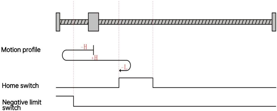
The present motor position is in the effective zone of the home switch. When homing starts, the home switch is at a high level, and homing is processed in the backward direction at a low speed. Homing stops when the motor reaches the falling edge of the home switch.
