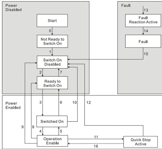
As shown in the diagram above, the state machine consists of three scenarios, namely Power Disabled, Power Enabled, and Fault.
