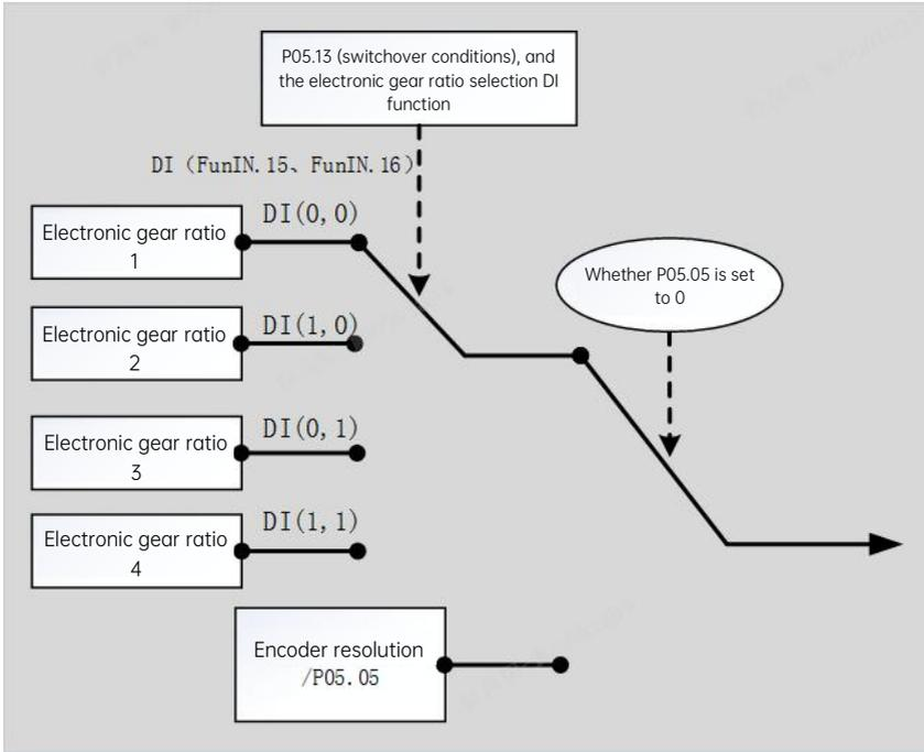
Fig. 5-2 Electronic gear ratio function diagram
