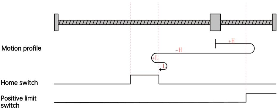
The present motor position is in the effective zone of the home switch. When homing starts, the home switch is at a high level, and homing is processed in the forward direction at a low speed till it reaches
