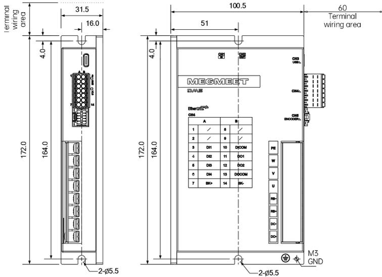
Fig. 2-2 SIZE B servo drive dimensions
