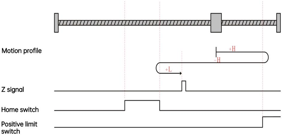
The present motor position is in the effective zone of the home switch. When homing starts, the home switch is at a high level, and homing is processed in the forward direction at a low speed. Homing stops when the motor reaches the rising edge of the Z signal.
