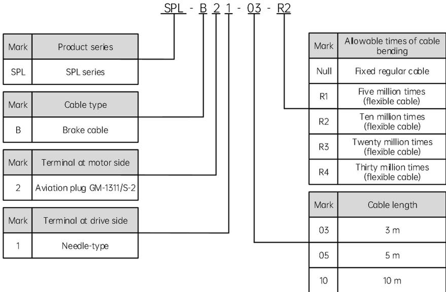
Fig. 1-9 Brake cable selection
