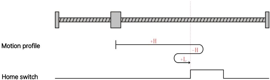
The present motor position is in the effective zone of the home switch. When homing starts, the home switch is at a high level, and homing is processed in the backward direction at a high speed till it reaches the falling edge of the home switch. Then, homing is processed in the forward direction at a low speed, and stops when the motor reaches the rising edge of the home switch.
