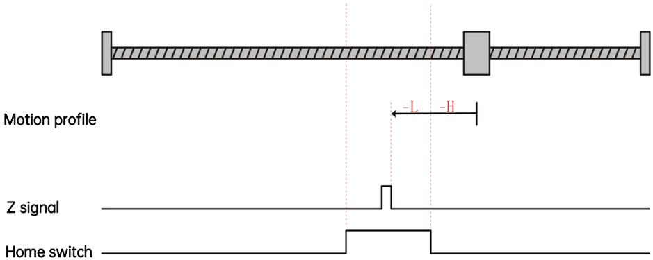
The present motor position is in the effective zone of the home switch. When homing starts, the home switch is a high level, and homing is processed in the forward direction at a high speed till it reaches the falling edge of the home switch. Then, homing is processed in the backward direction at a high speed till it reaches the rising edge of the home switch. Afterwards, homing continues in the backward direction at a low speed, and stops when the motor reaches the rising edge of the Z signal.
