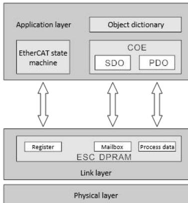
The EtherCAT (CoE) network reference model consists of two parts: the data link layer and the application layer.
