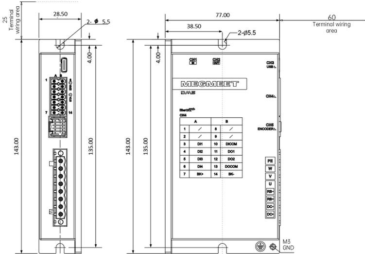
Fig. 2-1 SIZE A servo drive dimensions
