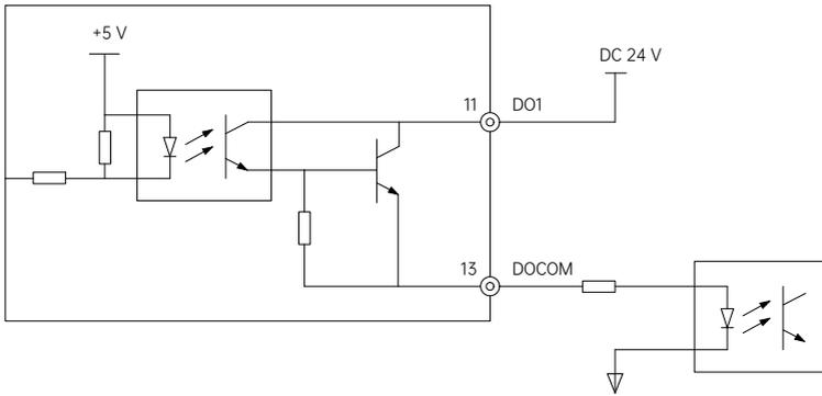
Fig. 4-8 DO terminal source (PNP) output wiring mode
