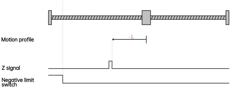
When the present motor position is at the Z signal, homing enable will be activated, the present position will be recorded as the home position, and homing will stop immediately.
