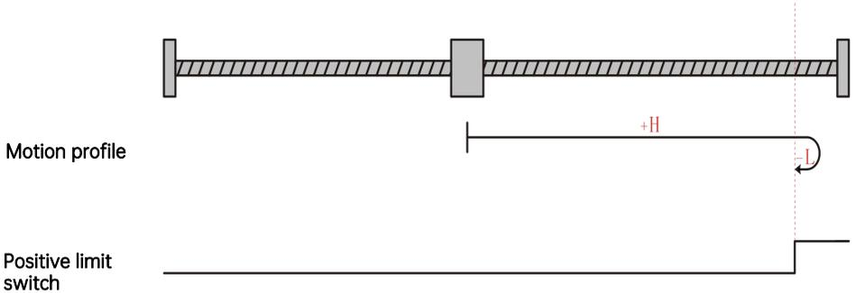
The present motor position is in the effective zone of the positive limit switch. When homing starts, the positive limit switch is at a high level, and homing is processed in the backward direction at a low speed. Homing stops when the motor reaches the falling edge of the positive limit switch.
