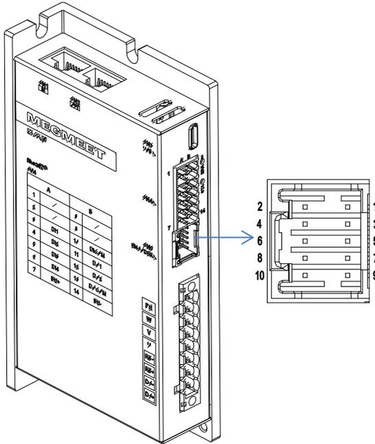
Fig. 4-1 Servo motor encoder signal connection diagram
