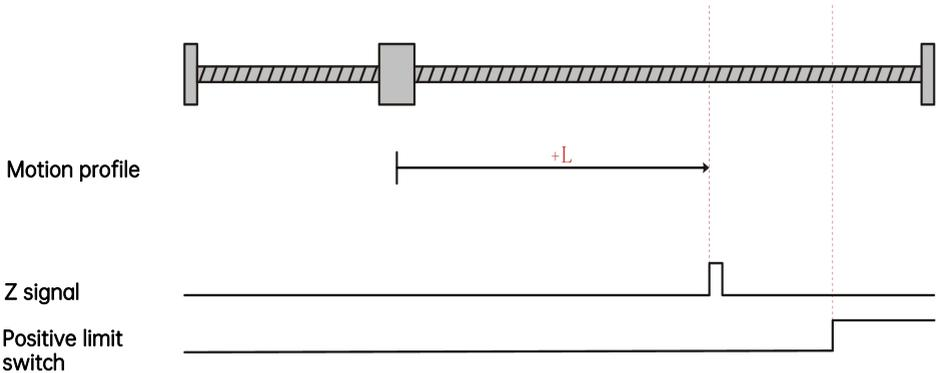
When the present motor position is at the Z signal, homing enable will be activated, the present position will be recorded as the home position, and homing will stop immediately.
