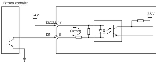
Fig. 4-4 NPN mode wiring of the DI terminal
