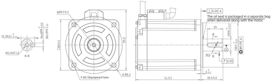
Fig. 2-6 Frame No. 80 servo motor dimensions (without brake)
