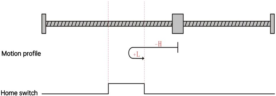
The present motor position is in the effective zone of the home switch. When homing starts, the home switch is at a high level, and homing is processed in the forward direction at a low speed. Homing stops when the motor reaches the falling edge of the home switch.
