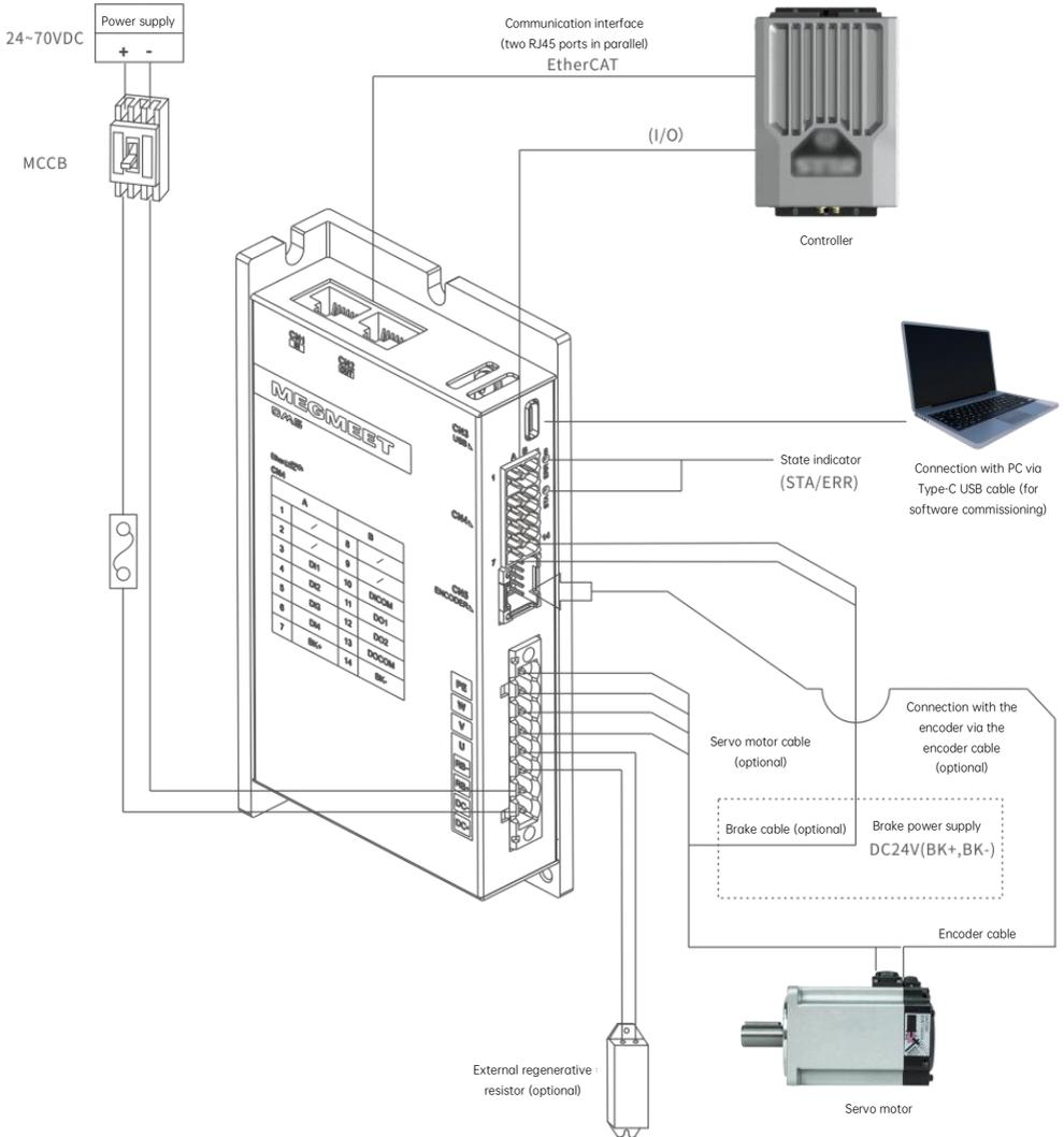
Fig. 3-2 SIZE A model wiring diagram
