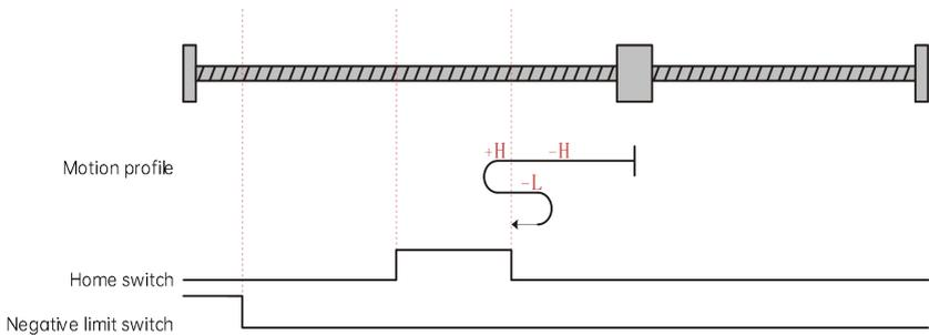
Fig. 6-10 Homing mode 1 motion profile Figure 3
