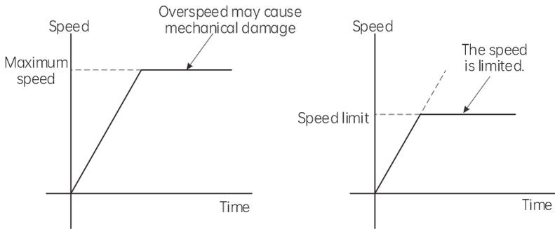
Fig. 6-34 Speed limit in torque control
