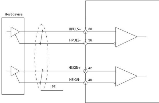
Fig. 4-15 High-speed pulse input wiring diagram
