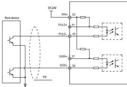
Fig. 4-13 Low-speed pulse reference NPN input wiring diagram
