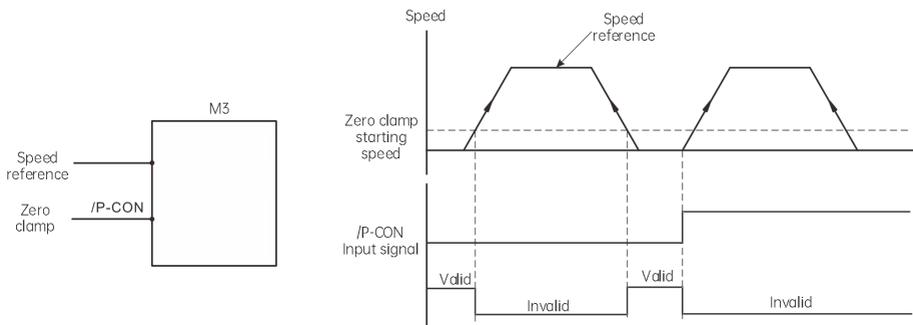
Fig. 6-32 Zero clamp logic
