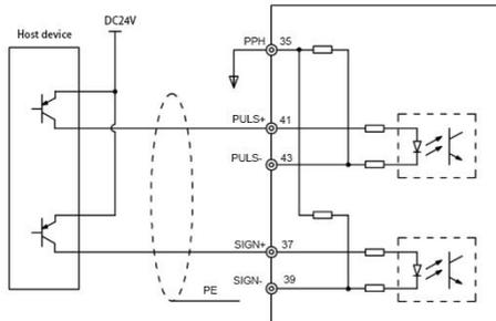
Fig. 4-14 Low-speed pulse reference PNP input wiring diagram
