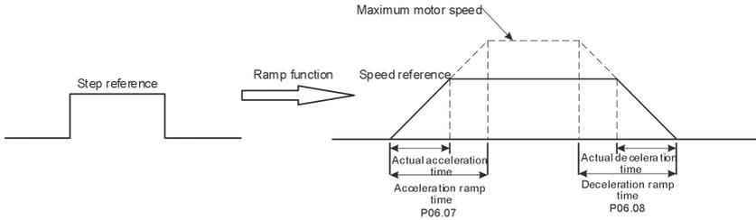
Fig. 6-31 reference ramp function operating logic
