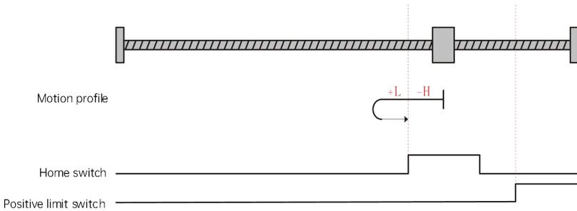
Fig. 6-6 Homing mode 0 motion profile Figure 2
