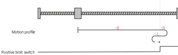
Fig. 6-21 Homing mode 6 motion profile Figure 1
