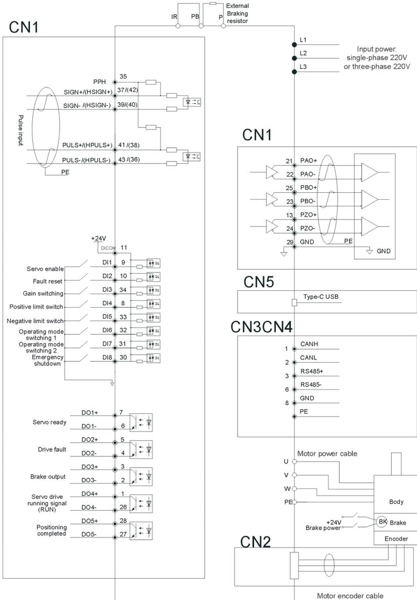
Fig. 6-1 Position control mode wiring
