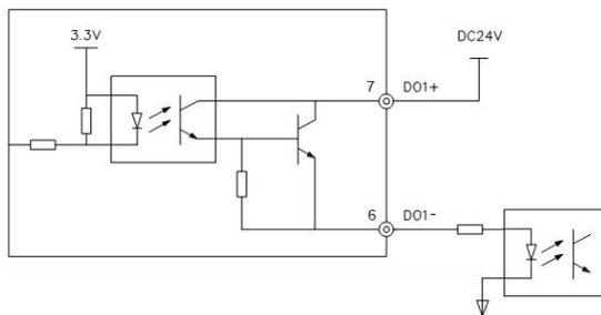
Fig. 4-11 DO terminal PNP (source) output wiring mode
