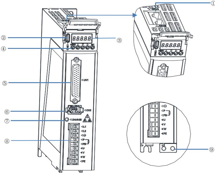
Fig. 1-5 Components of M3-P servo drive (M3-PS2R8A)
