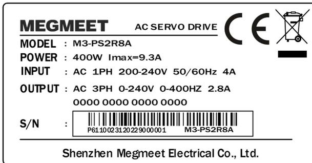
Fig. 1-4 Servo drive nameplate
