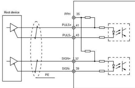
Fig. 4-12 Low-speed pulse reference differential input wiring diagram
