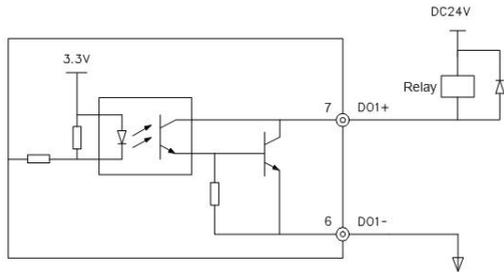
Fig. 4-9 DO terminal and relay wiring mode
