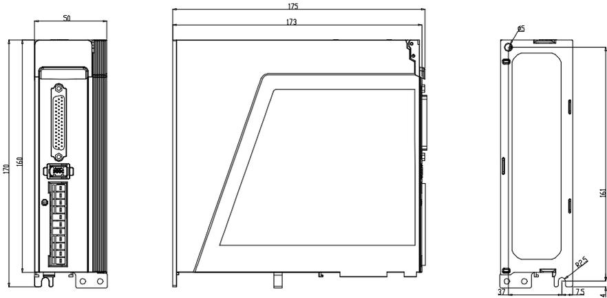
Fig. 2-2 SIZE B servo drive dimensions
