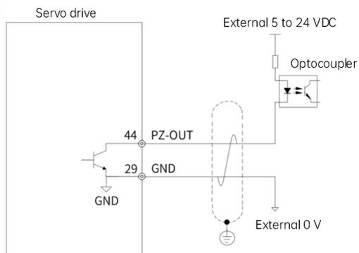
Fig. 4-18 Encoder frequency-division output wiring 3
