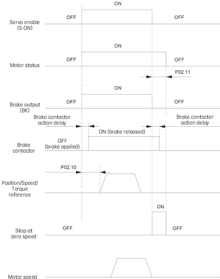
Fig. 6-37 Brake sequence for a motor at standstill
