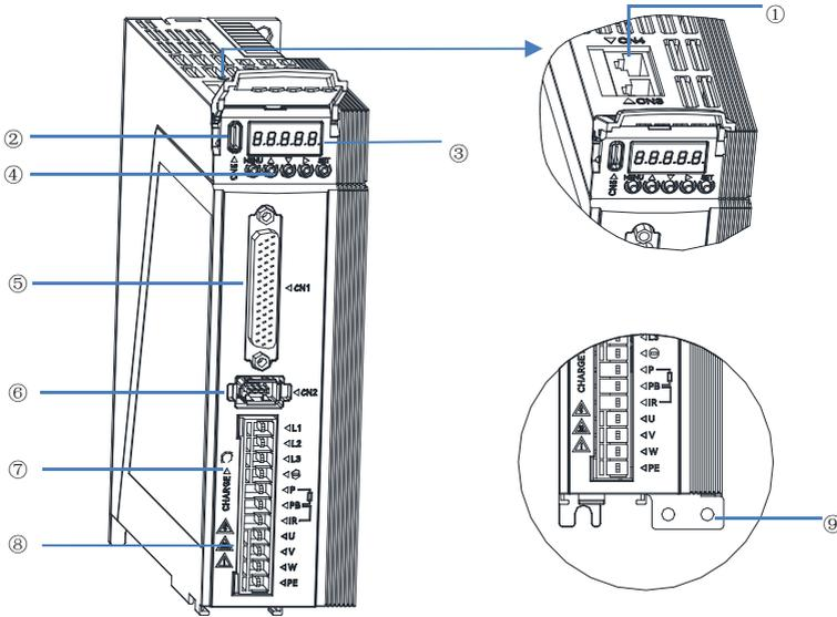
Fig. 1-6 Components of M3-P servo drive (M3-PS5R5A, M3-PS7R6A)
