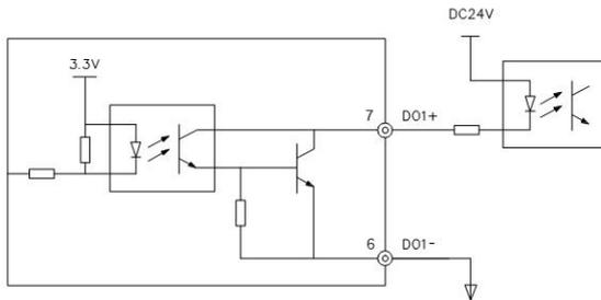
Fig. 4-10 DO terminal NPN (sink) output wiring mode
