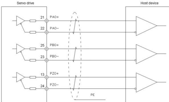
Fig. 4-16 Encoder frequency-division output wiring 1
