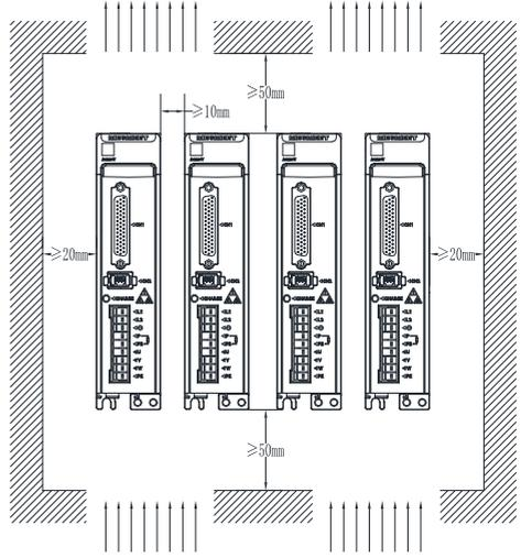
Clearance for side-by-side installation
