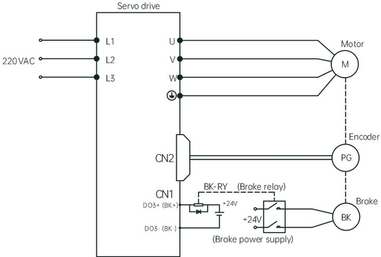
Fig. 6-36 Brake wiring diagram
