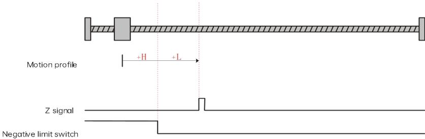
Fig. 6-28 Homing mode 9 motion profile Figure 2
