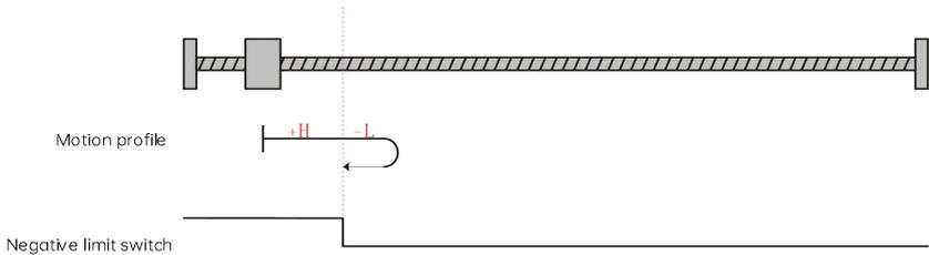
Fig. 6-24 Homing mode 7 motion profile Figure 2
