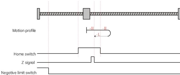
Fig. 6-19 Homing mode 5 motion profile Figure 2
