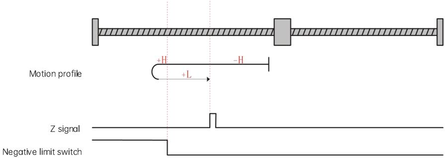
Fig. 6-27 Homing mode 9 motion profile Figure 1
