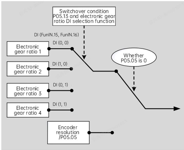
Fig. 6-4 Electronic gear ratio function diagram
