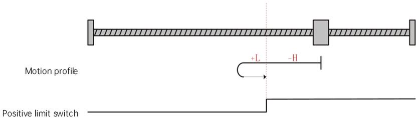
Fig. 6-22 Homing mode 6 motion profile Figure 2
