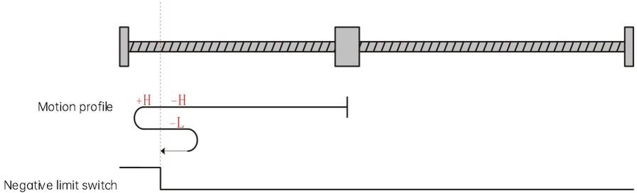
Fig. 6-23 Homing mode 7 motion profile Figure 1
