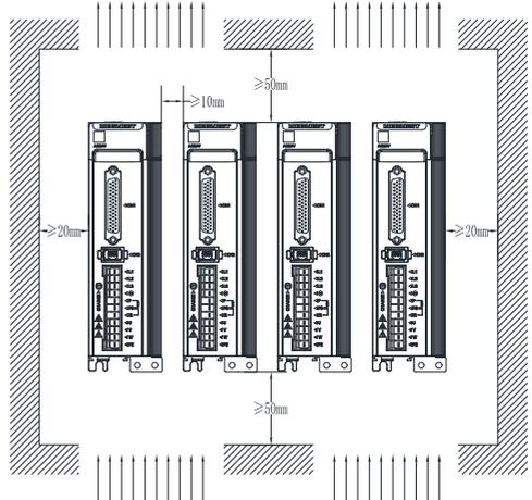
Clearance for side-by-side installation
