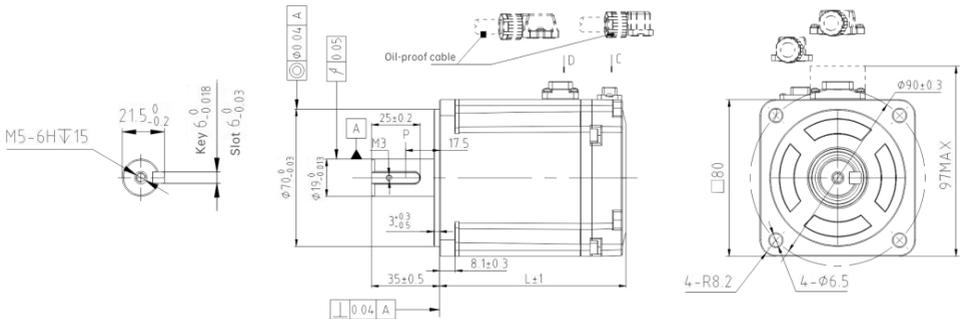
Fig. 2-4 Dimensions for 80 frame medium inertia straight plug economical servo motor (ST4-L series)
