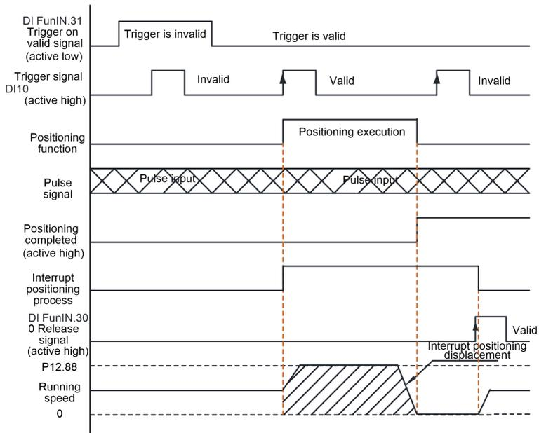
Fig. 6-29 Interrupt positioning sequence diagram
