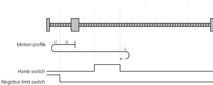
Fig. 6-8 Homing mode 1 motion profile Figure 1
