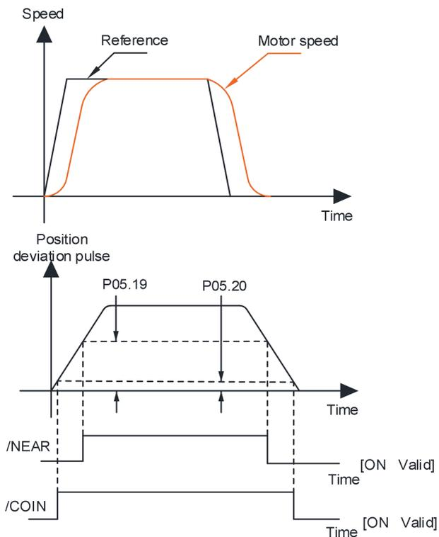
Fig. 6-2 Positioning near and positioning completed signal logic
