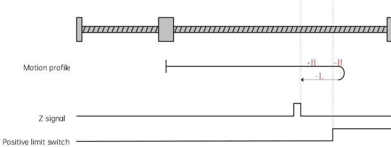
Fig. 6-25 Homing mode 8 motion profile Figure 1
