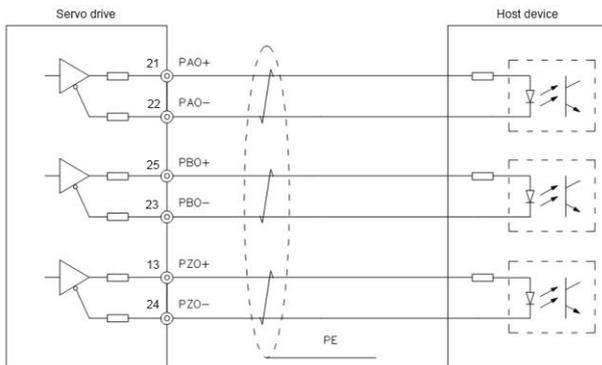
Fig. 4-17 Encoder frequency-division output wiring 2
