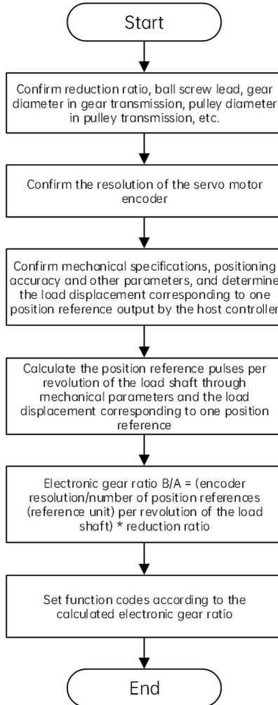
Fig. 6-3 Setting process of electronic gear ratio
