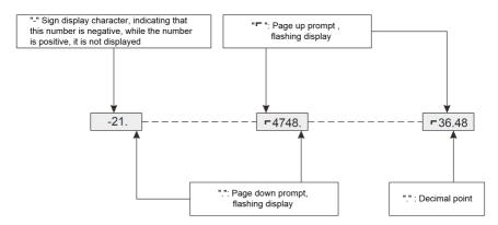
Fig.5-3 Parameter page display logic
