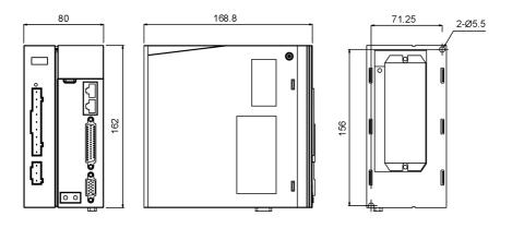
Fig.2-2 Dimensions for servo drive of SIZE B
