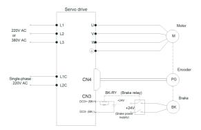
Fig.6-38 Brake wiring diagram
