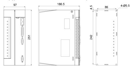
Fig.2-3 Dimensions for servo drive of SIZE C
