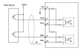
Fig.4-14 Low-speed pulse command PNP input wiring diagram
