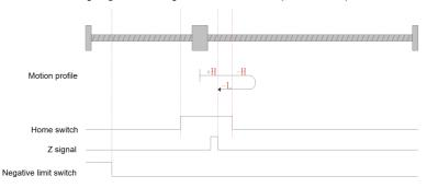
Fig.6-19 Homing mode 5 motion profile Figure 2
