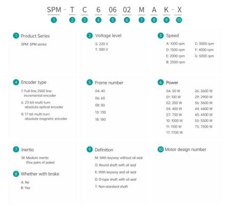
Fig.1-1 Servo motor model
