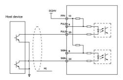
Fig.4-13 Low-speed pulse command NPN input wiring diagram
