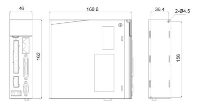
Fig.2-1 Dimensions for servo drive of SIZE A
