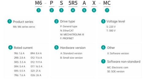
Fig.1-3 Servo drive model
