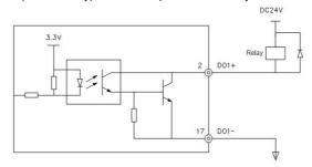
Fig.4-6 DO terminal connection relay wiring mode
