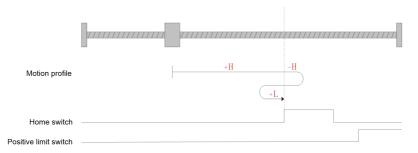
Fig.6-5 Homing mode 0 motion profile Figure 1
