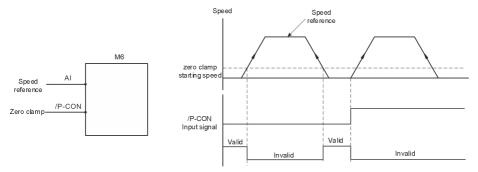
Fig.6-33 Zero clamp logic
