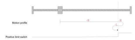
Fig.6-21 Homing mode 6 motion profile Figure 1
