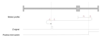
Fig.6-12 Homing mode 2 motion profile Figure 2
