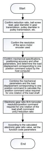
Fig.6-3 Electronic gear ratio setting process
