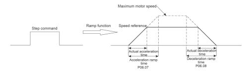
Fig.6-32 Command ramp function operating logic
