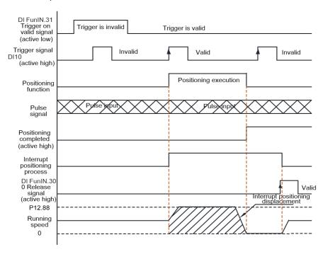
Fig.6-29 Interrupt positioning sequence diagram
