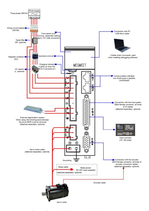
Fig.3-5 Three-phase 380V servo system wiring diagram
