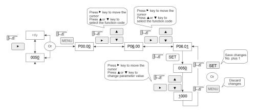
Fig.5-2 Working status display and parameter setting flowchart
