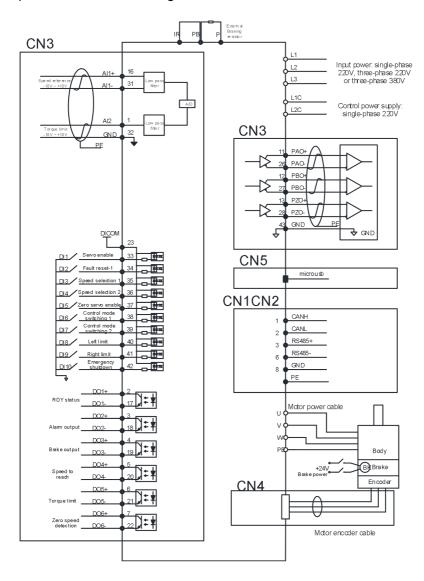
Fig.6-31 Speed control mode wiring
