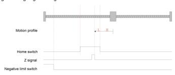
Fig.6-20 Homing mode 5 motion profile Figure 3
