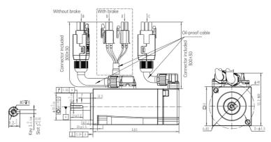
Fig.2-4 Dimensions for 40 frame medium inertia servo motor
