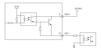
Fig.4-8 DO terminal source (PNP) output wiring mode
