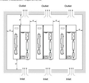
Fig.3-2 SIZE B/C servo installation diagram
