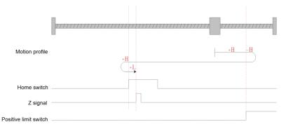
Fig.6-17 Homing mode 4 motion profile Figure 3
