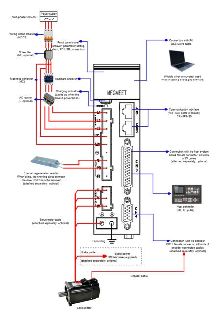
Fig.3-4 Three-phase 220V servo system wiring diagram
