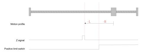
Fig.6-26 Homing mode 8 motion profile Figure 2
