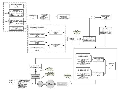
Fig.6-37 Function block diagram of torque control mode
