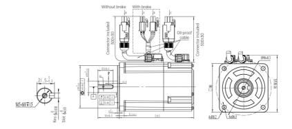
Fig.2-6 Dimensions for 60 frame medium inertia servo motor
