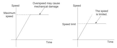
Fig.6-36 Speed limiter in torque control
