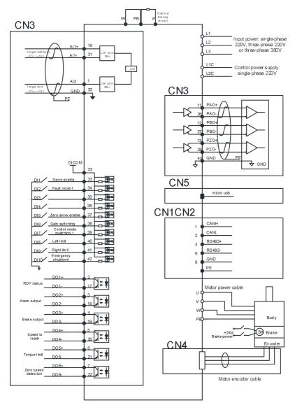
Fig.6-35 Torque control mode wiring
