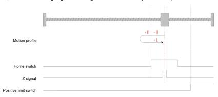
Fig.6-16 Homing mode 4 motion profile Figure 2
