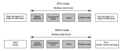
Attached Fig.1-1 Modbus protocol format
