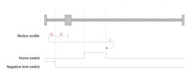
Fig.6-8 Homing mode 1 motion profile Figure 1
