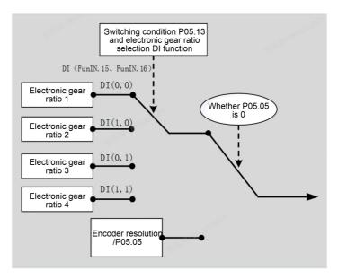
Fig.6-4 Electronic gear ratio function diagram
