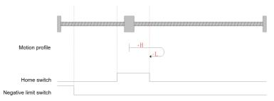
Fig.6-9 Homing mode 1 motion profile Figure 2
