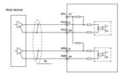
Fig.4-12 Low-speed pulse command differential input wiring diagram
