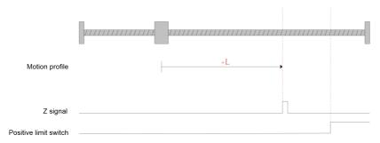
Fig.6-11 Homing mode 2 motion profile Figure 1
