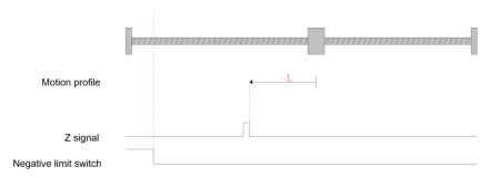
Fig.6-13 Homing mode 3 motion profile Figure 1
