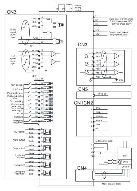
Fig.6-1 Position control mode wiring
