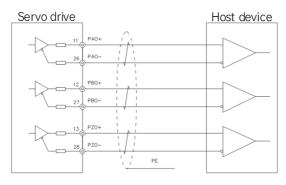
Fig.4-16 Encoder frequency dividing output wiring 1
