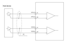
Fig.4-15 High-speed pulse input wiring diagram
