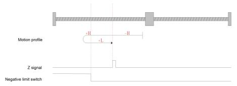
Fig.6-27 Homing mode 9 motion profile Figure 1
