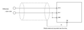
Fig.4-9 Al1 differential voltage input wiring diagram
