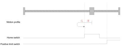
Fig.6-6 Homing mode 0 motion profile Figure 2
