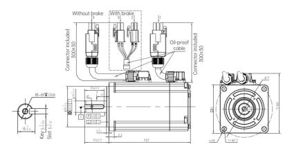
Fig.2-5 Dimensions for 60 frame medium inertia servo motor
