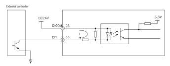
Fig.4-4 DI terminal NPN connection mode
