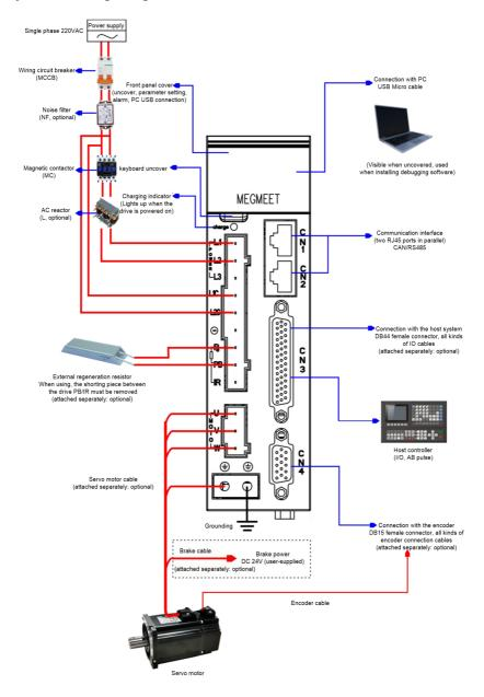
Fig.3-3 Single-phase 220V servo system wiring diagram
