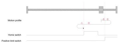
Fig.6-7 Homing mode 0 motion profile Figure 3
