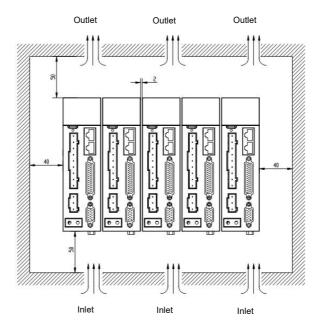
Fig.3-1 SIZE A servo installation diagram
