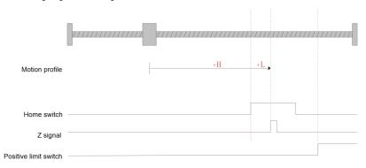
Fig.6-15 Homing mode 4 motion profile Figure 1
