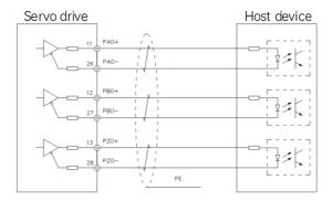
Fig.4-17 Encoder frequency dividing output wiring 2
