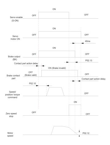
Fig.6-40 The brake timing when the servo motor is rotating
