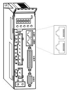
Fig.4-19 Communication interface connection diagram
